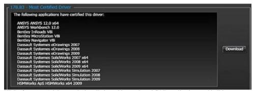
HP Performance Advisor tracks installed graphics cards and CAD applications and builds a database of vendor-certified device drivers.
