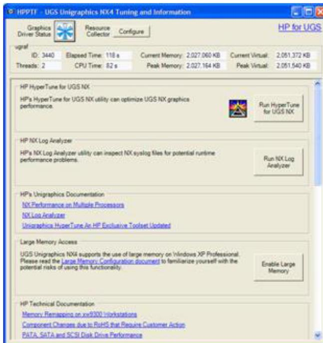
HP's Performance Tuning Framework (PTF) provides a Hyper Tune analyzer for each supported CAD application. By running the analyzer (at right, middle of screen), memory use and processor affinity can be set to allocate workstation resources to an application as desired.
