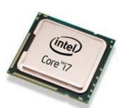
Figure 2. Intel's Core<sup>™</sup> i7 2920XM 2.50GHz chips provide Quad Core power, 32 GB of 1600Mz RAM capability and vPro turbo speeds of 3.50GHz.
