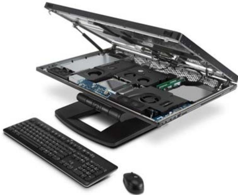
With tool-free serviceability, the interior of the HP Z1 is remarkably clear of cabling and electronics, allowing clean airflow through the vertical chassis. Hard drives and the standard optical drive drives are mounted flat on the rear of the chassis behind the display screen.
