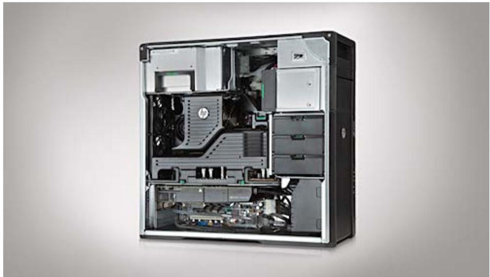
With tool-free serviceability, the interior of the HP Z620 is remarkably clear of all but the essential component cabling and has optimized air-flow management to allow lower speed and quieter fans.
