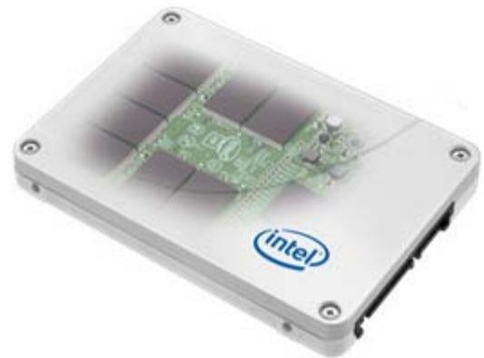
Figure 3. Externally, SSDs look like a hard drive, but inside they are all electronic with no moving parts.
