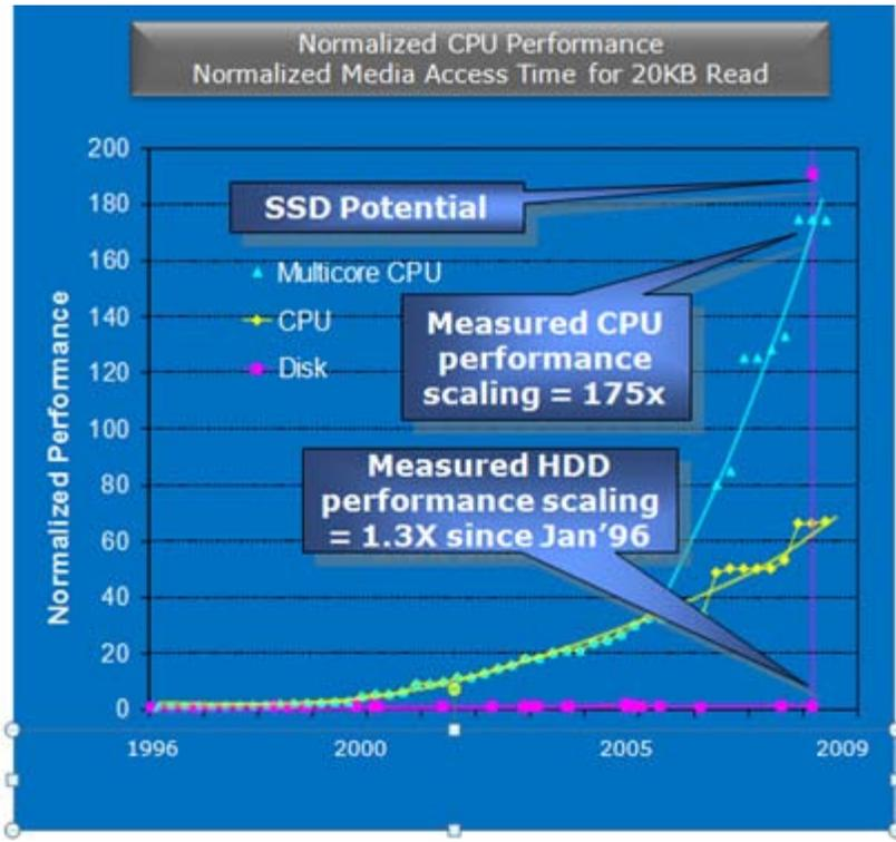
Figure 1. Compared to potential SSD performance, new multi-core CPU's hard drives are much slower.
