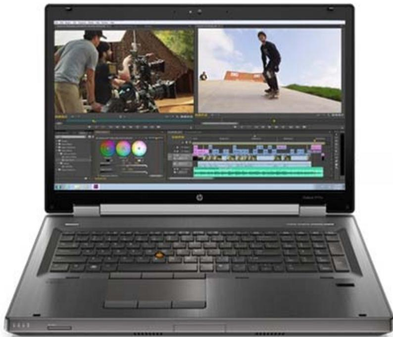
The HP Elitebook 8770w has a 17.3" diagonal screen size for compelling HD<sup>10</sup> displays even without a supported external display. Supporting 32 GB of RAM spread over four memory slots, the 3rd generation Intel® Core™ i5 or i7 processors yields desktop level computing power.<sup>1</sup>
