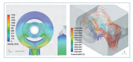
Figure 6: Sturman Industries designers relied on FloEFD for more than 80% of design for its Hydraulic Valve Actuation (HVA) product line. (Image courtesy of Sturman Industries)
