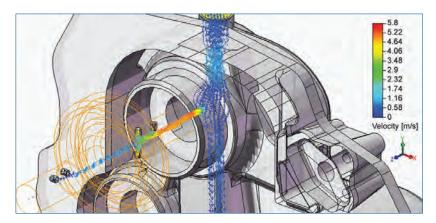
FloEFD, the industry's first concurrent CFD solution, embeds in leading MCAD environments and accepts device geometries directly.
