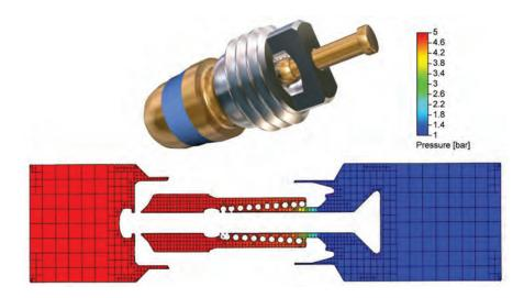
Figure 7: Ventrex Automotive used FloEFD to improve the flow rate of this CO<sub>2</sub> valve by 15%.
