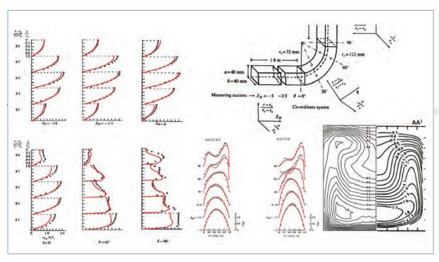
Figure 3: Velocity profiles at different cross-sections in different longitudinal planes. FloEFD validation and experimental results correspond closely in this example showing flow in a 90-degree bend of a 3D square duct.
