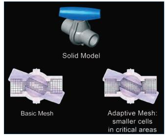
Figure 1: Using a rectangular adaptive mesh, the FloEFD concurrent CFD tool can automatically adjust cell size to deliver better resolution anywhere it is needed.
