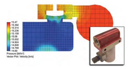
Figure 9: The original Shaw Aero Devices solenoid valve shown here exhibited a pressure drop of more than 6 psi. The Cut Plot shows the results of two design revisions that reduced the drop to about 1 psi. and subsequent revisions reduced the drop all the way to .71 psi, well within the customer's specifications. (Image courtesy of Shaw Aero Devices)
