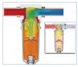
FloEFD handles challenging filter simulations with multiple filter modeling options, complex filter housings and comprehensive 3D visualizations.
