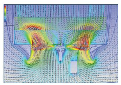
With its sophisticated multiple reference frame models, FloEFD can simulate complex fan characteristics, depict the flow and pressure fields surrounding a fan unit, and identify potential areas for improvements in energy efficiency and noise output. (Image courtesy of Bronswerk Heat Transfer BV).
