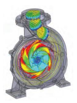
FloEFD can be used to determine pump efficiency and to optimize the design of components such as the housing, impeller, inlet and outlet sections. (Image courtesy of Johnson Pump).
