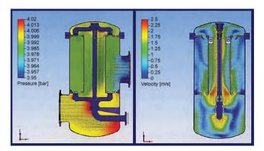
Figure 8: Boll & Kirch Filterbau GmbH uses FloEFD to simulate pressure losses so small that they would be very difficult to measure with a physical prototype.
