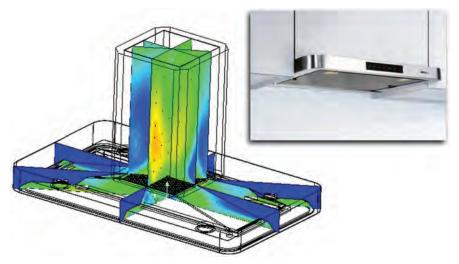
Figure 4: Marenco AG used FloEFD to design a new kitchen extractor hood for a client. The result is a hood that is not only more efficient that past designs but also operates at a lower decibel level than others, meeting the client's requirements. (Image Courtesy of Marenco AG)
