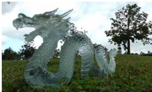
*Dragon Prototype - 3D Printed in Objet Clear Transparent Material*
