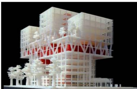
*Architectural 3D Model Printed on an Objet 3D Printer. Courtesy of Rietveld Architects.*
