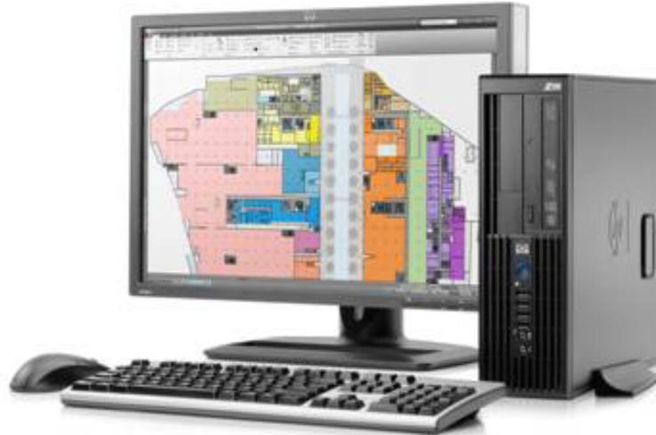
The Z200 Small Form Factor is 65% smaller than the Z200 Workstation and provides compact workstation-level performance by supporting only low-profile graphics boards
