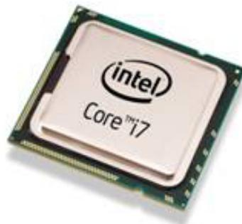
Intel's Core i7-720QM and i7-820QM chips provide quad-core power and 16-GB RAM capabilities for mobile workstations.
