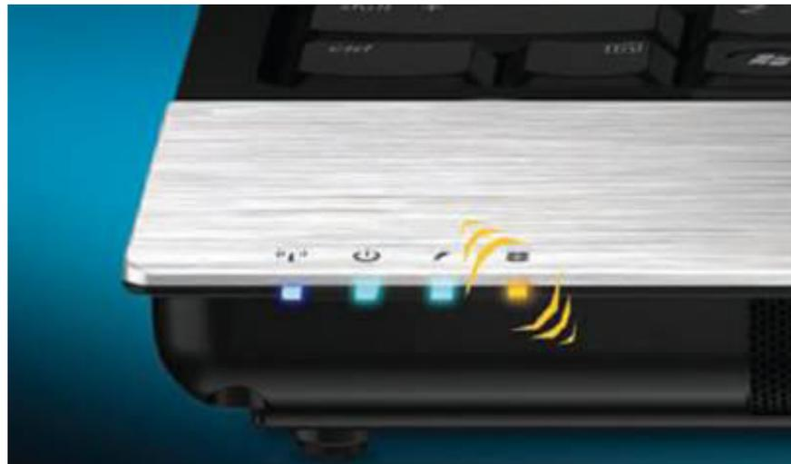
Workstations equipped with HP 3D DriveGuard have a hard-disk status light that indicates when your hard drive is parked, so you can move your workstation without worrying about data loss.
