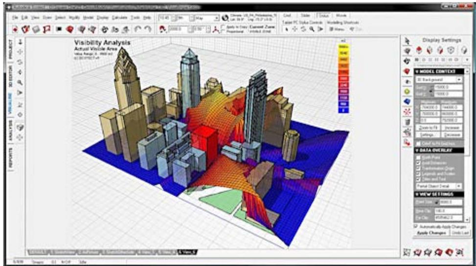
Applications such as visibility analysis bring a whole new dimension to building information modeling (BIM) design projects yet require more processing power to run in parallel with other applications. (Image courtesy of Autodesk)
