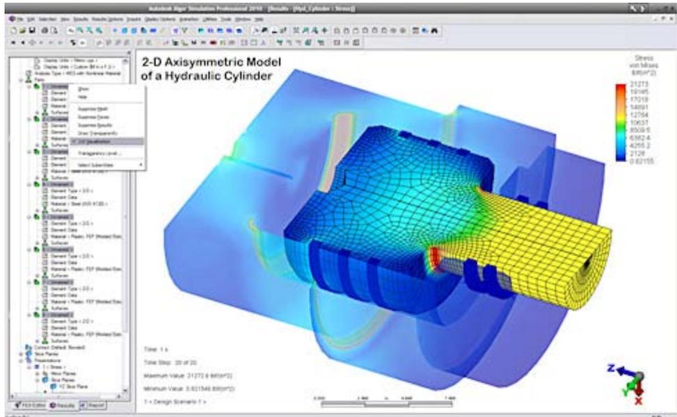
Applications such as finite element analysis allow simulation of loads to run concurrently with other design applications to let you examine more "What if?" design scenarios. (Image courtesy of Autodesk)
