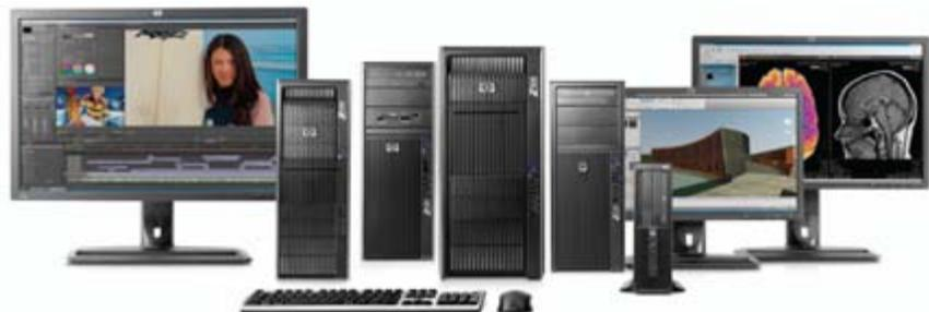
The HP Z210 CMT Workstation and HP Z210 SFF Workstation (at right) have front accessible drive bays but otherwise maintain front accessible USB and FireWire ports and vertical pipe styling like their siblings the HP Z800, HP Z600, and HP Z400.
