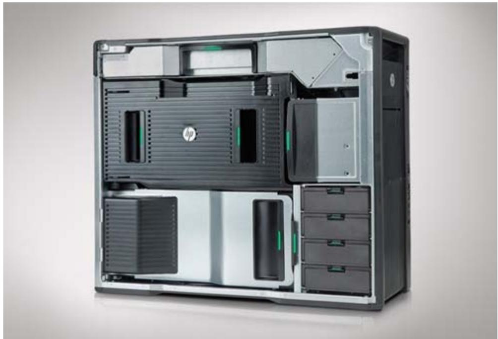
The HP Z820's internal air guides move cooling air through the chassis to achieve optimum cooling allowing processors to run faster.
