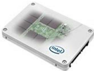
The solid-state drive, an option on the new HP Z230s, consists entirely of memory, which functions much faster than a mechanical hard drive — especially helpful in data-intensive CAD applications.
