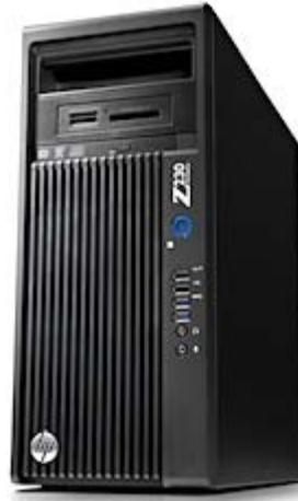
The Z230 Tower has front-accessible drive and media reader bays plus a variety of USB 2.0/3.0, FireWire, and audio ports. It opens to expose substantial internal options for video cards and additional drives — all accessible without tools.
