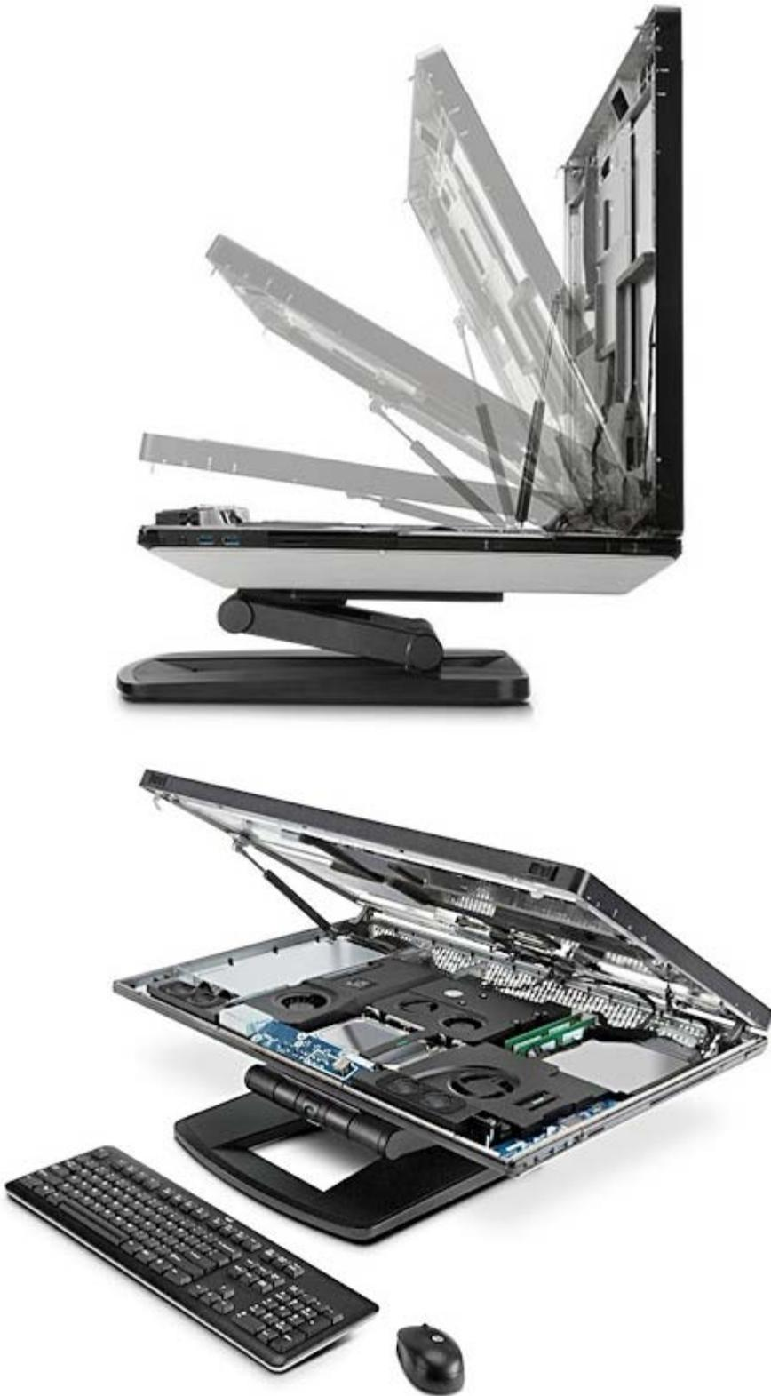
As easy to open as the hatch of your car, the HP Z1 G2 reveals an easy to customize, tool free internal chassis with room for expansion drives, RAM, and graphics card.
