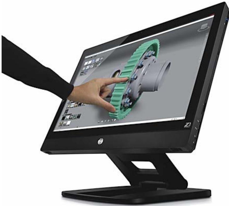
HP's Z1 G2 looks like a thick-bezel standalone monitor; closer examination reveals ports around the perimeter and rear of the unit. Screen image courtesy of Autodesk.
