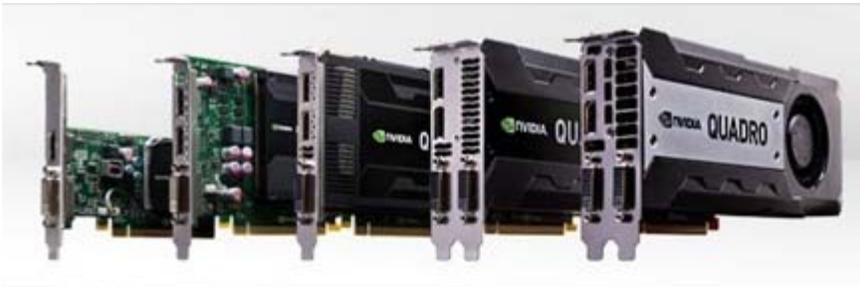
Different graphics cards have different sizes, slot requirements, and interface outputs. (Image credit: NVIDIA Corp.)
